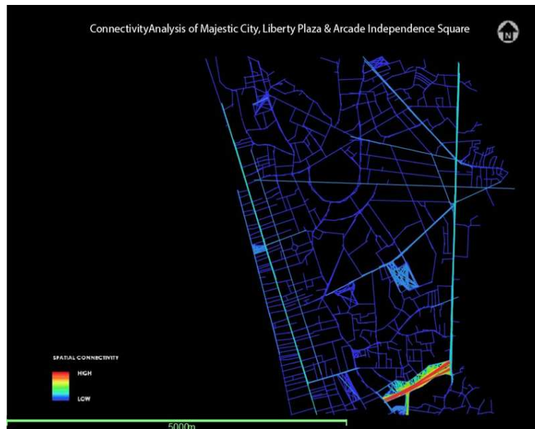
Figure 7 Connectivity analysis of MC, LP & AIS (Source: Compiled by author by using Space Syntax software)
