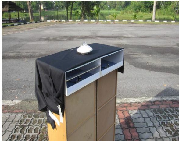
Fig. 8 Daylight measurement using Delta OHM LP-PHOT 01 with data loggers for internal illuminance and Delta OHM LP-PHOT 02 with data logger for external illuminance.
