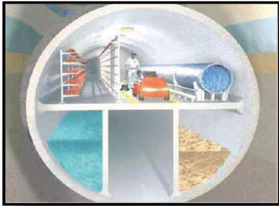
Figure 8: Utilidors in Turkmenistan Source: ITA-AITES (2012)
